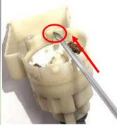
Push in the direction of the arrow. XThis photo is taken with the board removed, but it actually shows the direction of the screwdriver
