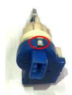
2.Lift the three claws with a flathead screwdriver and remove the base.
