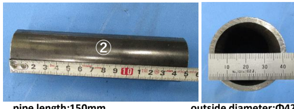
pipe length:150mm (similar alternatives are acceptable) outside diameter:Φ42
