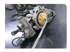
(4)Using SST, remove the vane pump pulley from the vane pump drive shaft.
